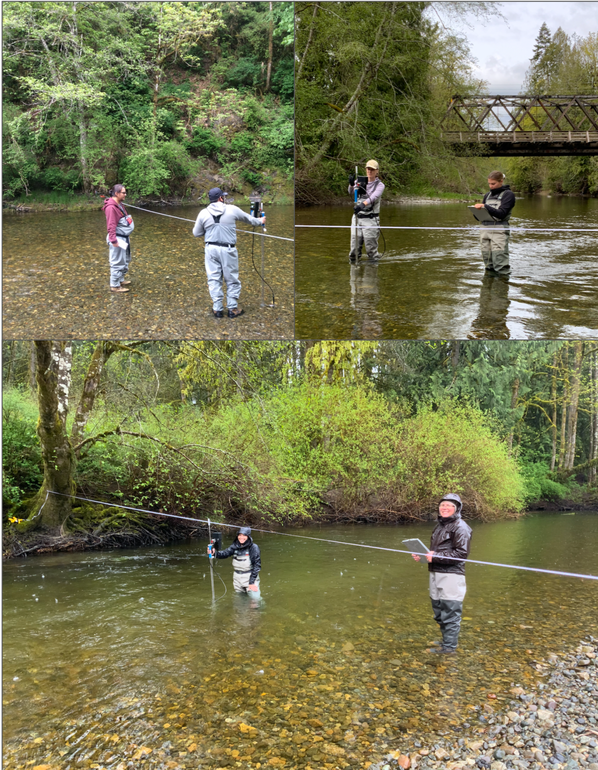
Photo 4-1. Koksilah River EFA survey flow measurements.
